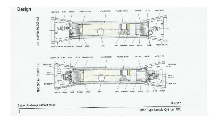
Right angle needle valves with ¼"NPT female port connections are fitted to 10,000-psi cylinders. A special is fit into the sample side which allows for evacuation of the cylinder.
